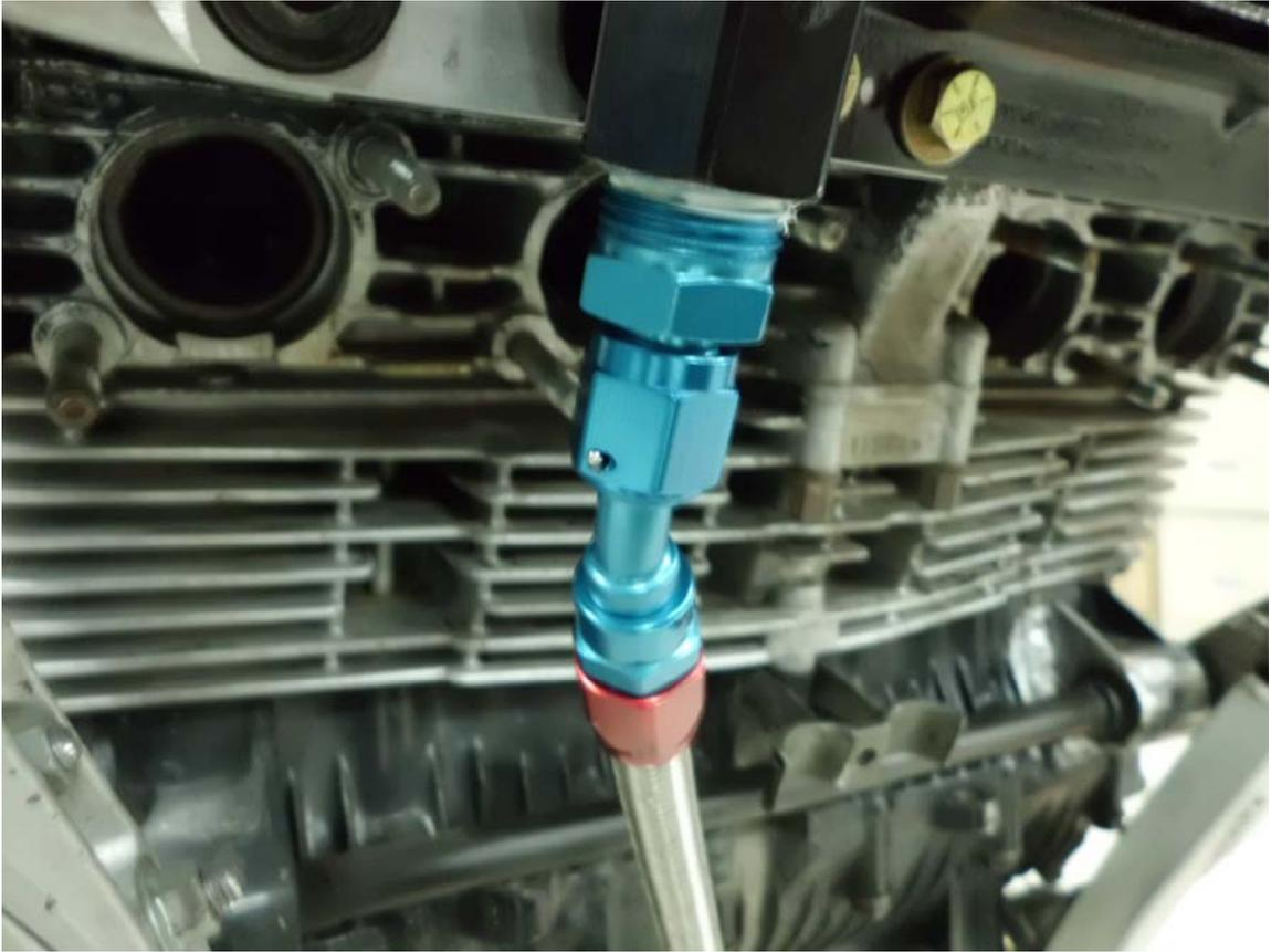
24) The fitting are a swivel design fitting that will allow you to rotate each respective hose end for proper alignment to the respective fitting.
