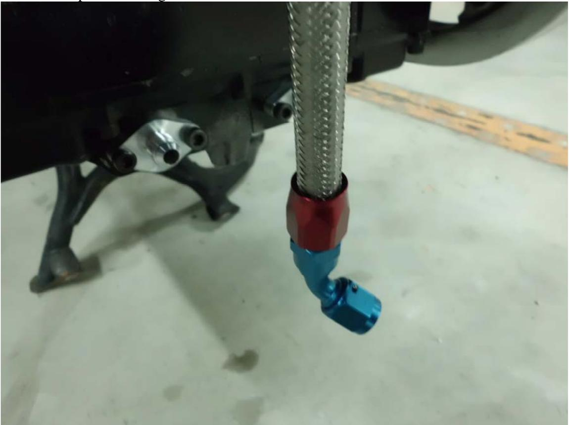
25) Once the lower hose fitting is aligned with the oil pan fitting, add a drop or two of clean oil to the threads and seat and install hand tight.
