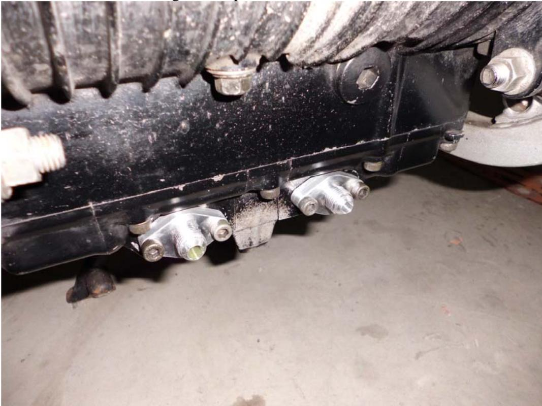
22) On the 84-90 the oil line run in front of motor mount cross tube. 92+ the oil lines should run behind the motor mount cross tube.
