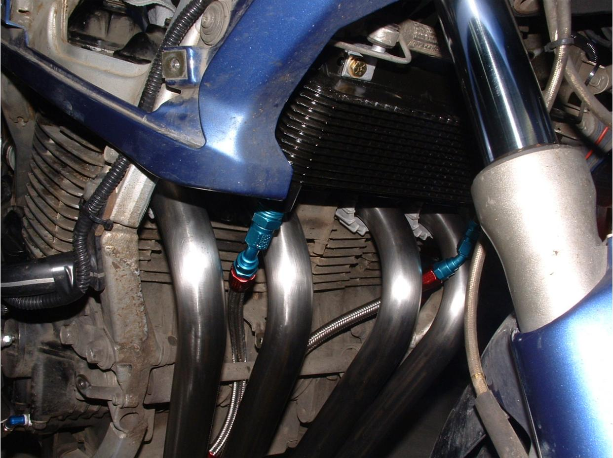
23) Note the oil lines have a 30 and 60 degree fitting on the end of each hose. The 30 degree or less sharp curved fitting attaches to the oil cooler add a drop or two of clean oil to the threads and seat and install hand tight. The hoses should be curve to the center of the bike.
