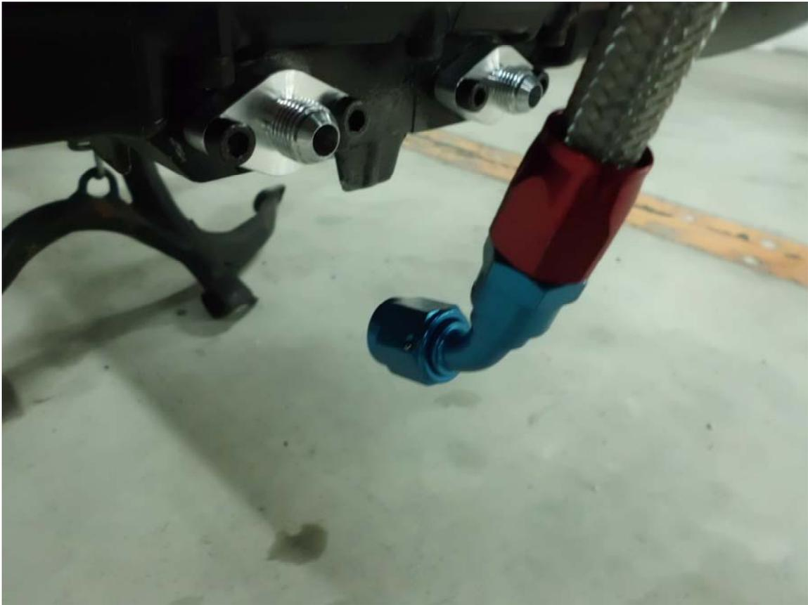
26) A/N fittings are designed to seal via the taper seat in each fitting and **NO** Teflon tape or pipe dope should be used on the threads. The use of Teflon tape or will promote over-torque of the fitting resulting in damage.
