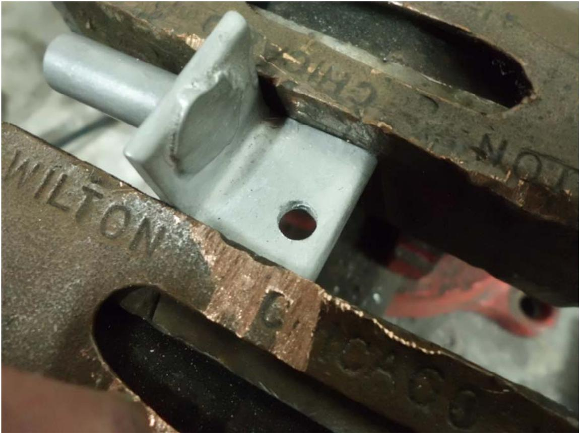
17) Mount the, now drilled, upper cooler brackets to the front of the upper mounting flange and tighten the bolts until there is just enough movement to move the bracket for alignment purposes.
